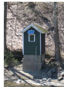
Figure 3 A stream gauge on the Kinderhook Creek, in Stockport, NY. A typical stream gauge records the water flow in cubic feet per second at 15 to 60 minute intervals. The data is electronically transmitted to USGS offices every 1 to 4 hours.
