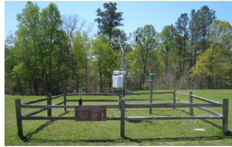
Figure 2 A weather station in the Taskinas Creek watershed near Williamsburg Virginia. This station measures wind direction and speed, temperature, humidity, atmospheric pressure, solar radiation, and precipitation.
